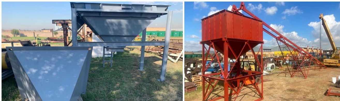
Figure 3 & 4 – Crusher Feed Hopper fully manufactured and DMS Feed Conveyor and Hopper Fabricated in South Africa
