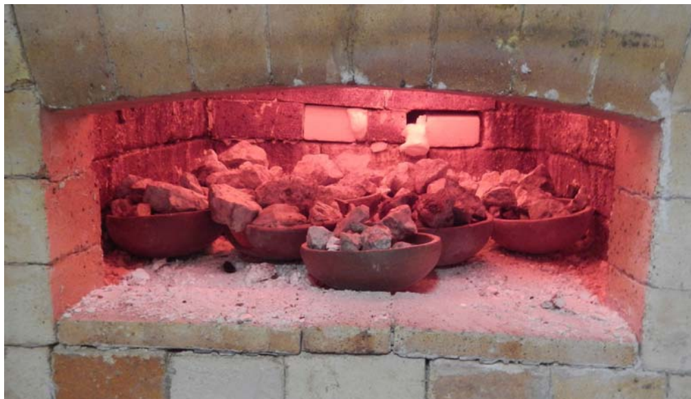
Figure 4 – Decrepitation Furnace (100kg per day at 1080C)
