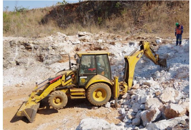
Blasted Main Pegmatite ready for stockpiling
