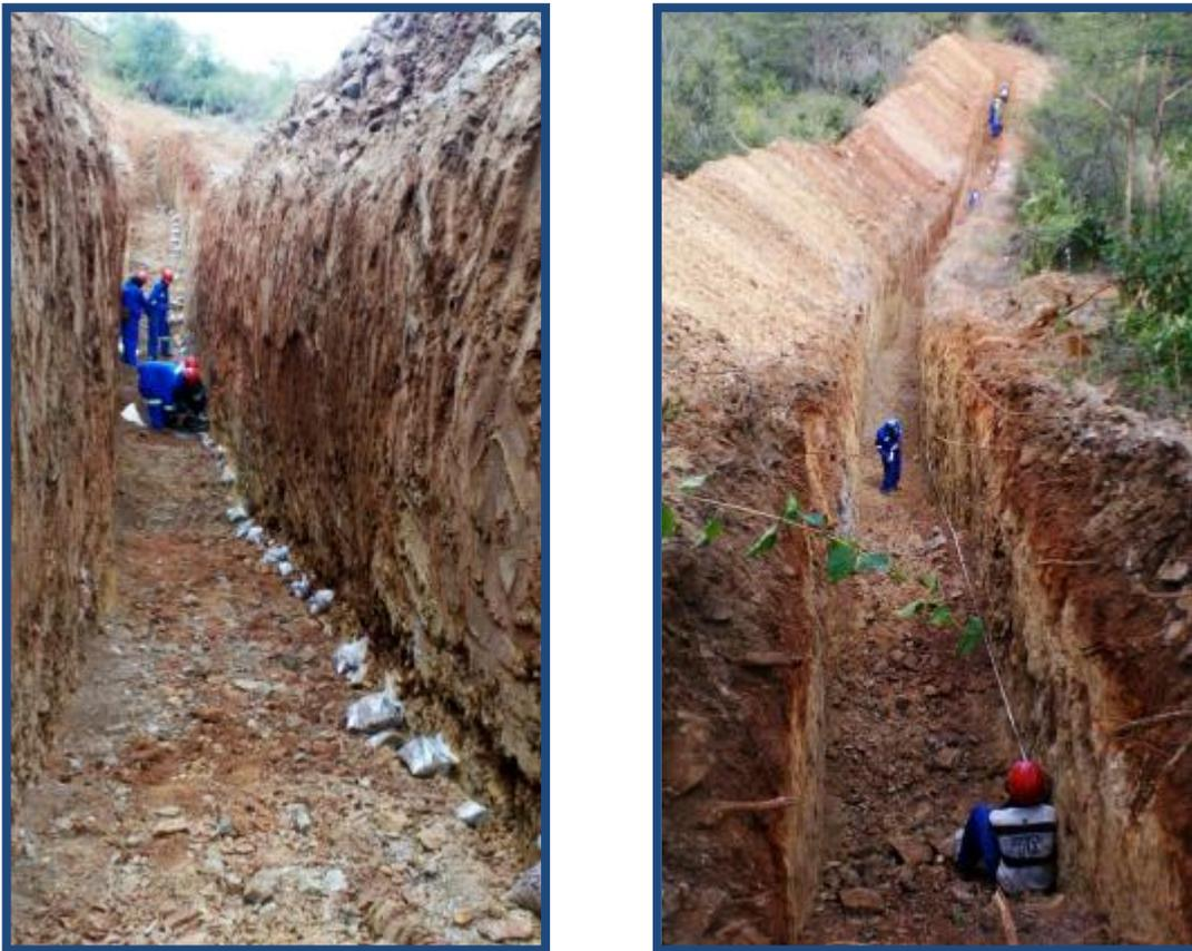
Figure 1: Photos of trench sampling
