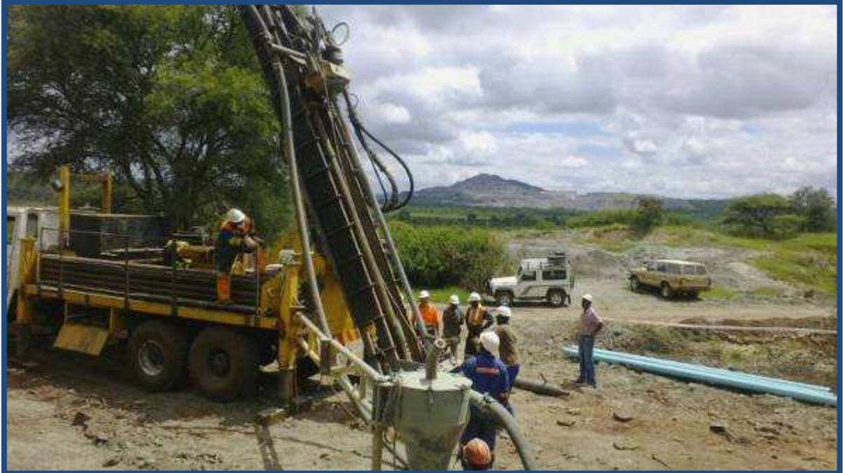
**A Super Rock 5000 RC rig of Ox Drilling, beginning hole BPC1 at Prestwood.** In the immediate background is the old tailings dump, whilst to the north in the background is the Colleen Bawn PPC limestone quarry
