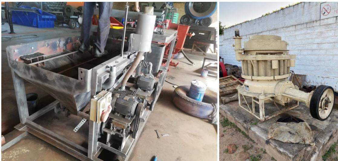
**Figure 3 & 4 – DMS unit undergoing modifications and refurbishment in South Africa and Cone Crusher refurbished in South Africa, factory acceptance tested in Zimbabwe**
